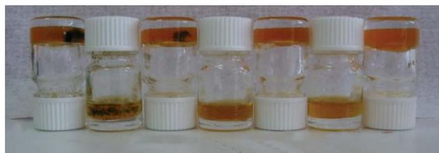
**Fig. 1** Organogels **1**-SWCNTs obtained from **1** and containing decreasing amounts of SWNTs (1, 0.5, 0.2, 0.1, 0.05, 0.02, and 0.01% w/w, respectively from left to right) (from ODCB).
